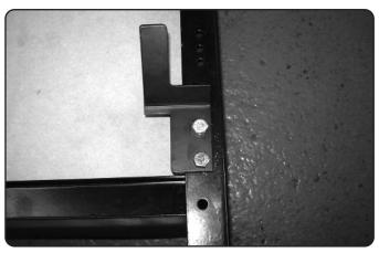
Loosely fix brackets to the back of the seat frame using nuts and bolts only.
