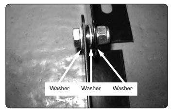
Assemble the base frame to the back frame using nut/bolt and three washers as shown in picture.
