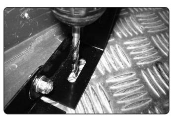
NOTE - Beware of electric cables when drilling holes Hook seat back into mounting points at the top then slide the base backwards until the baseplate is flat with the vehicle body. Drill a 6.5mm hole at each end and bolt down the seat assembly to the vehicle.
