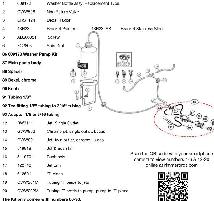
Numbers 1-6, 12-20 are listed to provide information useful in completing the installation of TR4-4A.
