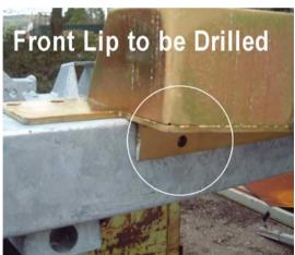
There are another 2 holes that need to be drilled. These are on top of the bumper where the winch is to be positioned. It may be necessary to enlarge the other bolt holes depending on the winch application.
