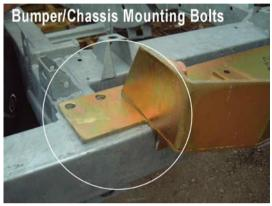
The lip, with 2 bolt holes, on the winch mount should now be in front of the bumper. Drill the bumper and bolt.
