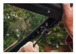
30. Set about refitting the gas struts (new units are recommended), the internal plastic lock cover and, last but not least, the wiper arm.
