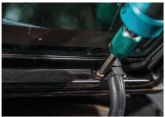
2. Unscrew the heated screen wiring covers, then disconnect connectors. The right-hand side may have wiring for the central locking actuator.
