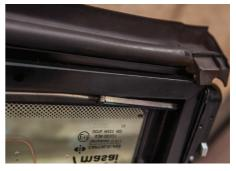
27. When the catches lock and unlock easily, refit the internal covers. Once covered, you won't be able to fettle with the rods any longer.
