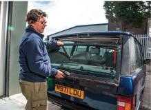
21. You need one person to hold the tailgate, and another for the screws. The trick for fitting the screws involves two small screwdrivers.
