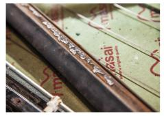
15. The seal will probably be grubby and have rust flakes stuck to it. Give it a careful wire brush and then scrub clean to prepare it for refitting.
