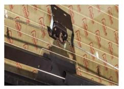
19. Next, connect the catch actuator rods, and drill the covers. Leave the covers off, as you will need to access the rod locknuts later.
