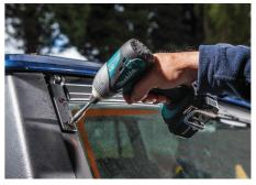
5. Undo the four tailgate screws, and remove the tailgate. We needed an impact driver to persuade my rusted bolts to move.
