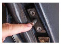
25. The catch plates on the body are adjustable, and the pegs offset. The plate may need turning around to get the peg in the right place for the new tailgate.
