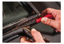
12. Remove the handle, the strut mounts, and the lower rubber seal. The seal is no longer available, and the one part you definitely should avoid damaging.
