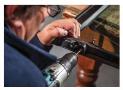
8. Be prepared to have to drill out most of them. A small pilot hole will make accurate drilling easier a second time with a larger drill bit.
