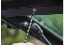
29. When the catches lock and unlock easily, refit the internal covers. Once covered, you won't be able to fettle with the rods any longer.
