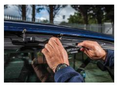
1. Remove the wiper arm, then soak the four tailgate hinges liberally in penetrating fluid.
