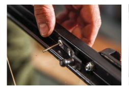
20. Finally, set about refitting the gas strut mounts using the rivets provided. The tail-gate is now ready to refit onto the vehicle.
