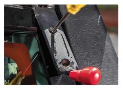
23. Next, lower the hinge down to the tailgate, and then insert another screwdriver through the top holes of the hinge, tailgate and floating plate.
