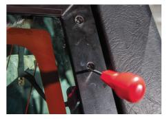
22. First of all, carefully insert one screwdriver into the lower hole, ensuring it goes through the floating plate inside, too.
