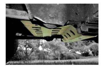
Check to ensure for clearance and then fully tighten all bolts.
