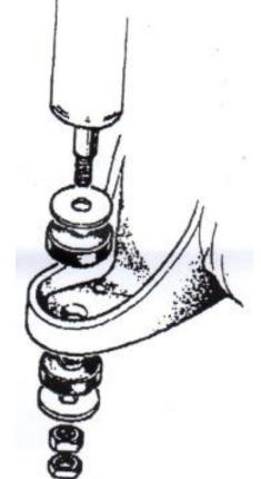
ASSEMBLE THE DAMPER INTO THE TRAILING ARM – USE THE LOCK NUTS TO SECURE.
