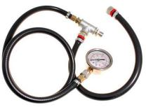
This test gauge assembly compromising required male and female 3/8<sup>th</sup> BSP connections plus stainless steel glass fronted pressure damped gauge is rquired to accurately test the fuel pressure setting on the above systems.
