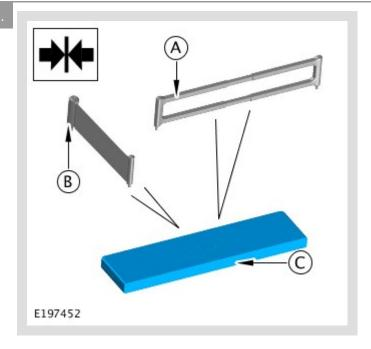
When not in use, compress the beam and band assembly and place in the transport bag enclosed with the kit.
