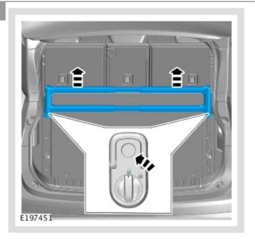
To remove the beam and band assembly, unlock the loadspace sliding D-loops and then lift the component upwards.
