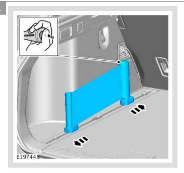
Move the band assembly to the desired position while holding down the button on top.
