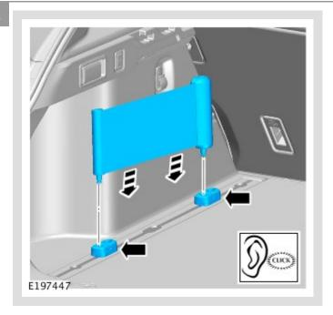
Attach band assembly to the chosen sliding D-loops.
