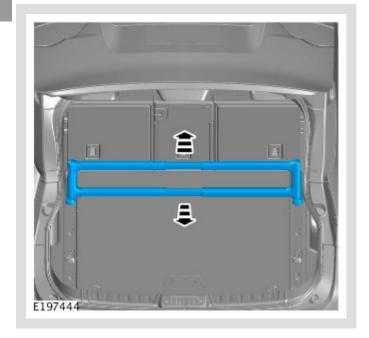
Move the beam assembly to the desired position.
