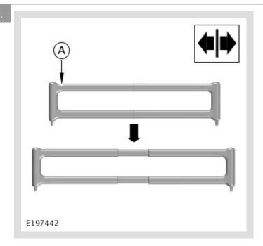
Expand the beam assembly.
