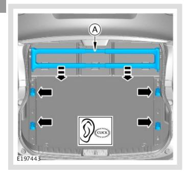
Attach beam assembly to the chosen sliding D-loops.
