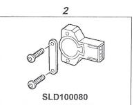
NOTE: Throttle Position TP sensor kit SLD100080 will for a short time contain a TP sensor with internal spring fitted, this sensor can be fitted to aluminium throttle housings without concern. The kit is also common with plastic throttle housing applications, for this reason a spreader plate has been included, if fitting to aluminium throttle housings the spreader is not required.
